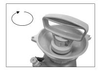
Unlock the handle and pump at least 30 times or until the pressure relief valve opens;
